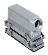
Complete connector, CSZ series, composed of 2 spring terminal connection inserts with 24 poles + PE, and bulkhead mounting housing with 2 levers and hood with side cable entry
