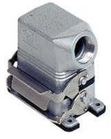
Complete connector, CNZ series, composed of 2 screw terminal connection inserts with 10 poles + PE, and bulkhead mounting housing with 1 lever and hood with side cable entry
