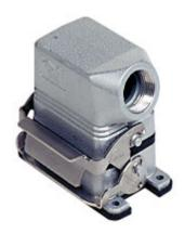
Complete connector, CNZ series, composed of 2 screw terminal connection inserts with 6 poles + PE, and bulkhead mounting housing with 1 lever and hood with side cable entry
