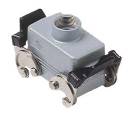
Hood, C-TYPE series, with 2 levers, M32 top cable entry, size "57.27", high construction, without gasket
