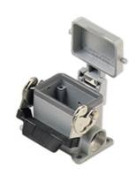
Surface mounting housing, EMC series, with 1 lever, M32 x 2 cable entry, size "44.27", high construction, with metal cover
